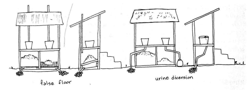
This design uses one side at a time to allow the other side to compost
