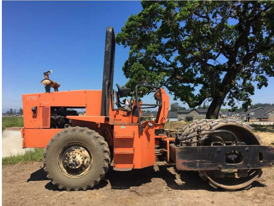
Figure 35. Sheepfoot roller used to compact sandy-silt soil.
