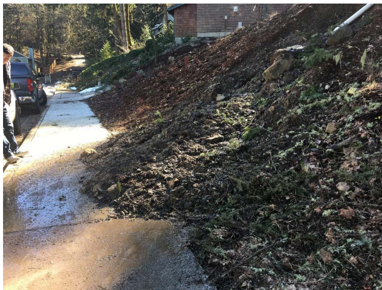
Figure 15. Slope failure due to excess ground moisture.
