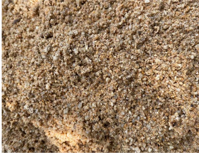
Figure 4. Soil matrix of a well-graded sand.
