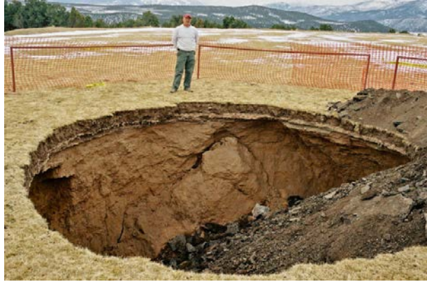
Figure 25. Ground subsidence in loess deposits (courtesy of Colorado Geological Survey )
