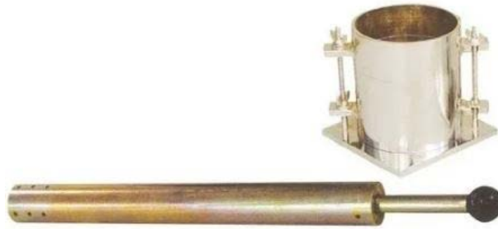
Figure 37. Proctor Test Equipment - Hammer and Mold
