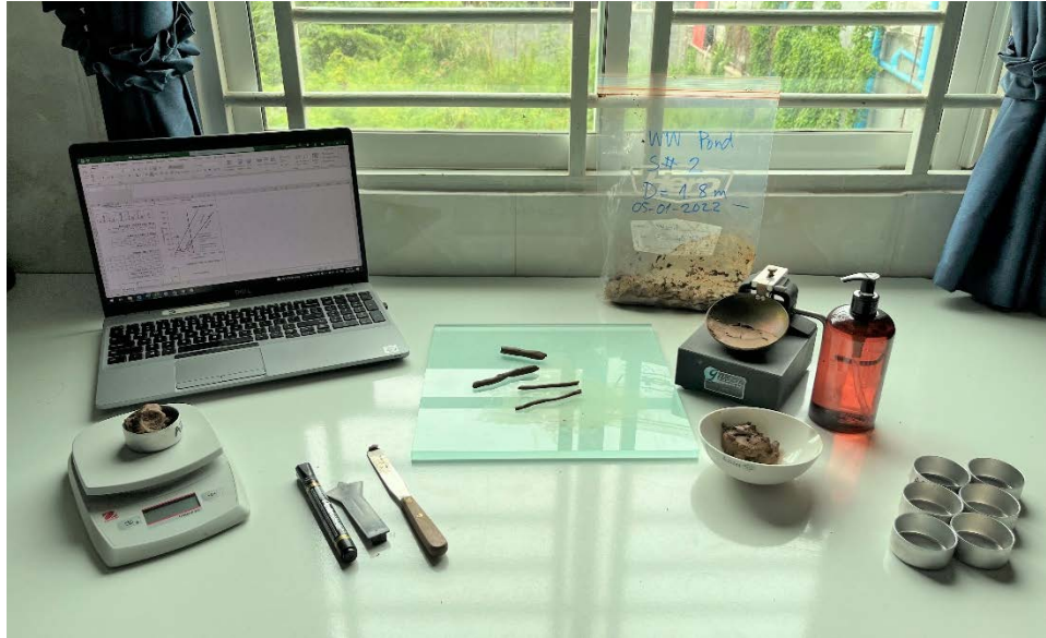
Figure 8. Typical Atterberg limit testing setup.
