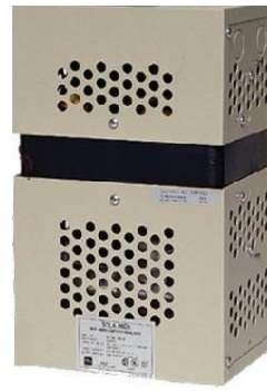
Figure 29. The transformer is operated so that its magnetic circuit is somewhat saturated, and this provides the near constant voltage at the output.
