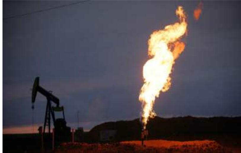
Methane flaring to reduce greenhouse gas
