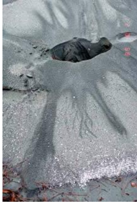
Figure 23. Sand boil exposed at the ground surface (courtesy of USGS )
