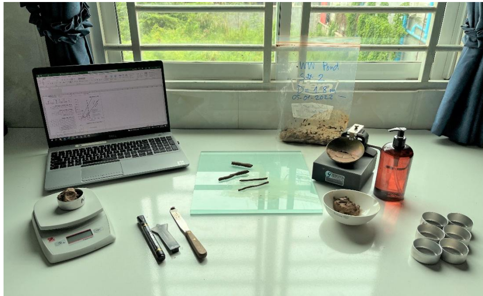
Figure 8. Typical Atterberg limit testing setup.
