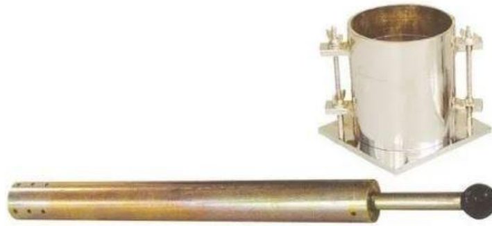
Figure 37. Proctor Test Equipment - Hammer and Mold
